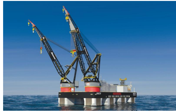
Obr 3 2x10 000mt Tub Crane [1]
